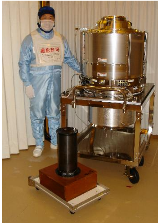
Figure 6: Photograph of microlithographic lenses developed in 1987 (Black) and 2004 (Silver)
