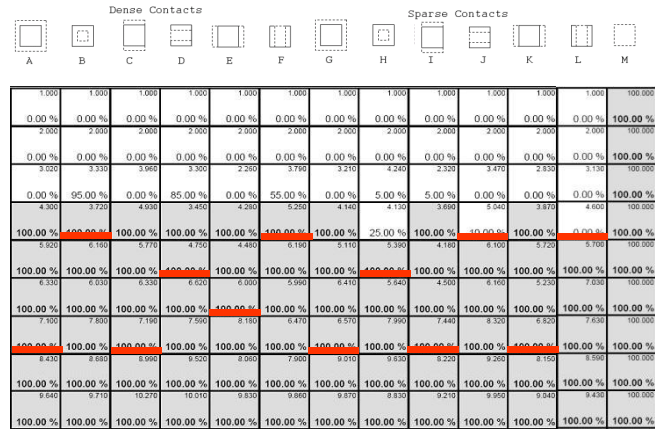
Figure 4-3: Die-to-database contact flux sensitivity with 125nm pixel transmitted illumination from Cetus-600-193
