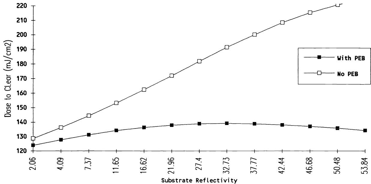
Figure 3 Effect of PEB on E0 variation from PROLITH/2 simulations using the input parameters listed in Table I.
