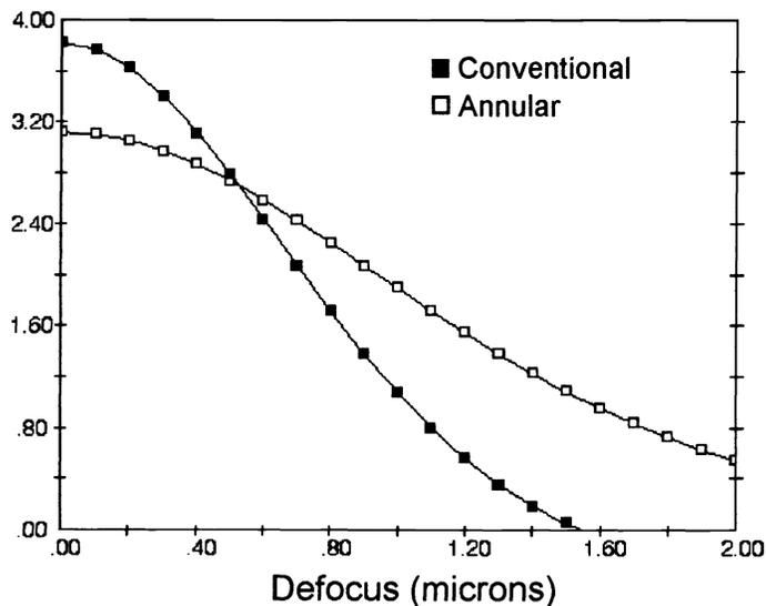
Figure 5. Comparison of annular and conventional illumination for  $0.35\ \mu\text{m}$  isolated lines with i-line,  $\text{NA} = 0.52$ . The conventional illuminator uses  $\sigma = 0.5$ , and the annular illuminator has a center  $\sigma$  of 0.5 with a width of 0.1.
