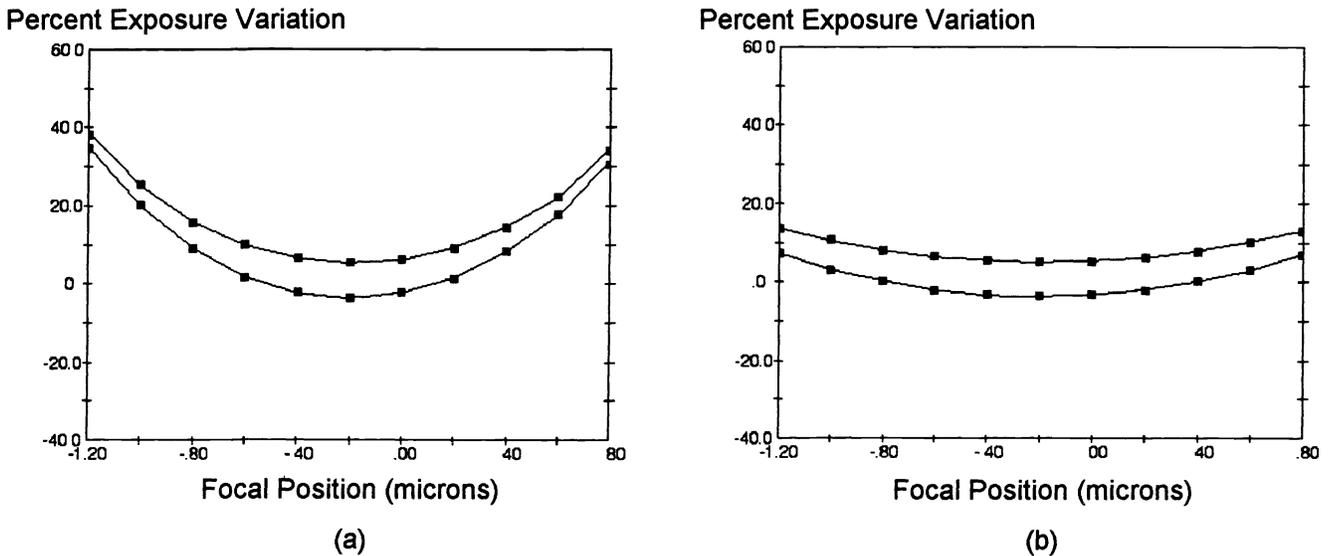
Figure 7. Comparison of the focus-exposure process windows for a) conventional illumination and b) annular illumination for 0.35 μm equal lines and spaces with i-line, NA = 0.52. The conventional illuminator uses  $\sigma = 0.5$ , and the annular illuminator has a center  $\sigma$  of 0.5 with a width of 0.1. Contours are for  $\pm 10\%$  linewidth specifications. (Simulated with PROLITH/2.)
