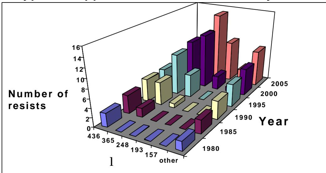
Figure 1. Growth in the number of different resists offered by a typical supplier since 1980, grouped by exposure wavelength.
