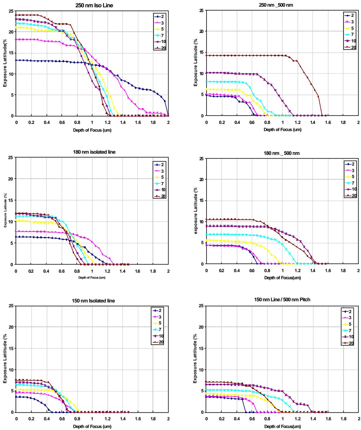
Figure 5. Comparison of exposure latitude versus DOF plots for 250, 180, and 150 nm features on 1000 and 500 nm pitch. Develop contrast value as indicated.
