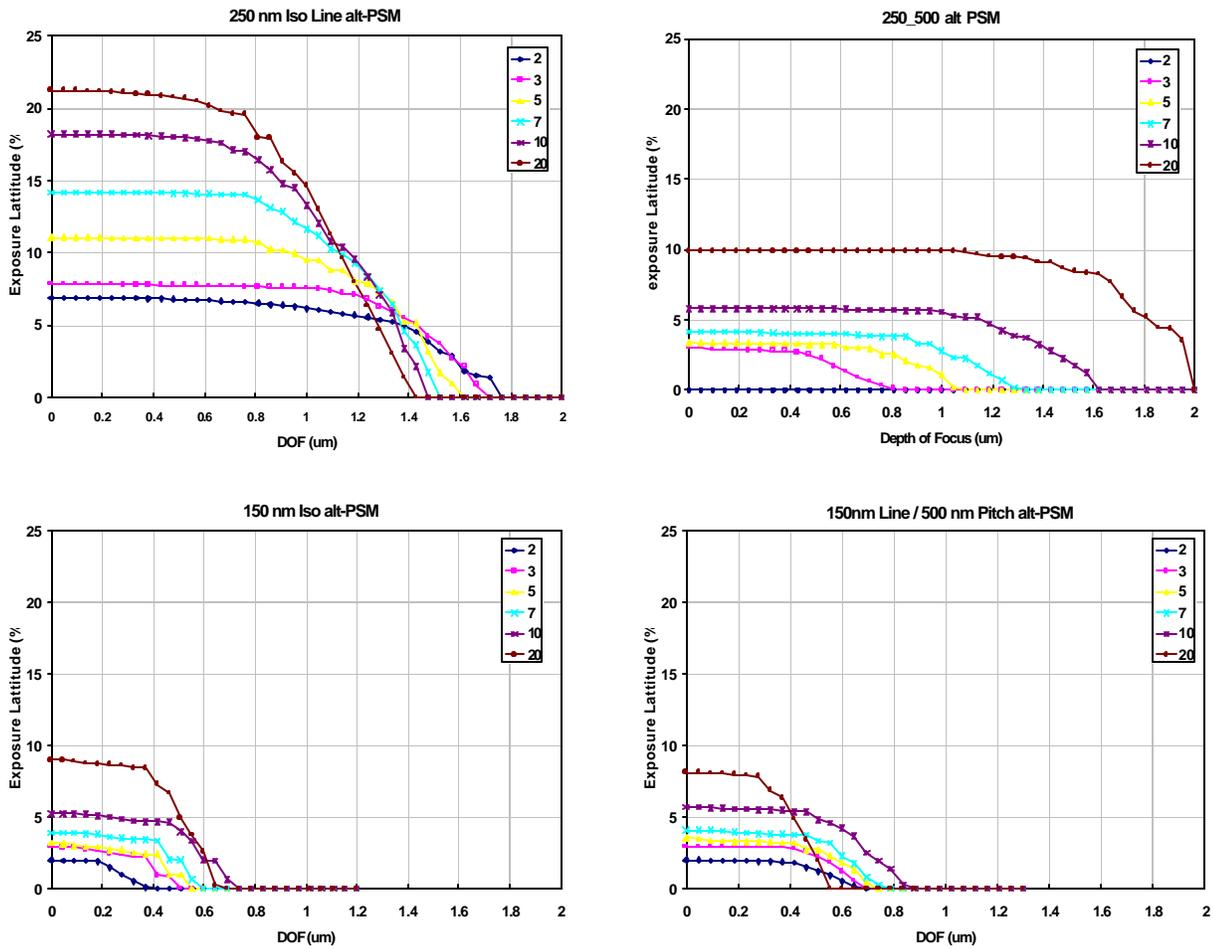
Figure 8. Comparison of exposure latitude versus DOF plots for 250 and 150 nm features on 1000 and 500 nm pitch using alternating phase shift exposure at NA = 0.50 and sigma = 0.30.
