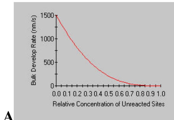
Figure 3. Dissolution rate profiles for the two resists.
