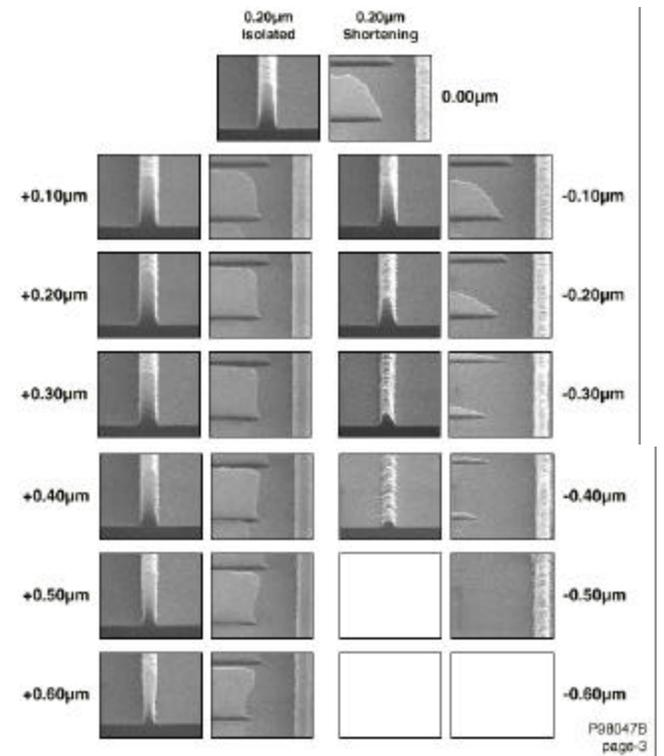
Figure 4. SEM photographs corresponding to the SEM data in Figure 2. Top = Resist B, Bottom = Resist A.
