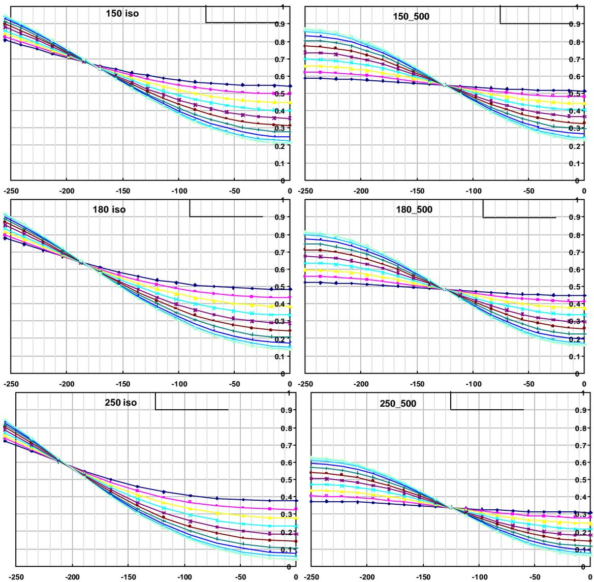
Figure 6. Aerial images through focus corresponding to the lines from Figure 4. Edge of chrome is shown at top of each graph. X axis is mask position, Y axis is light intensity.
