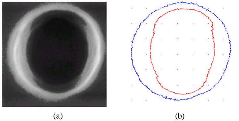
Figure 4. The processed image (a) used to detect the inner and outer edges (b).
