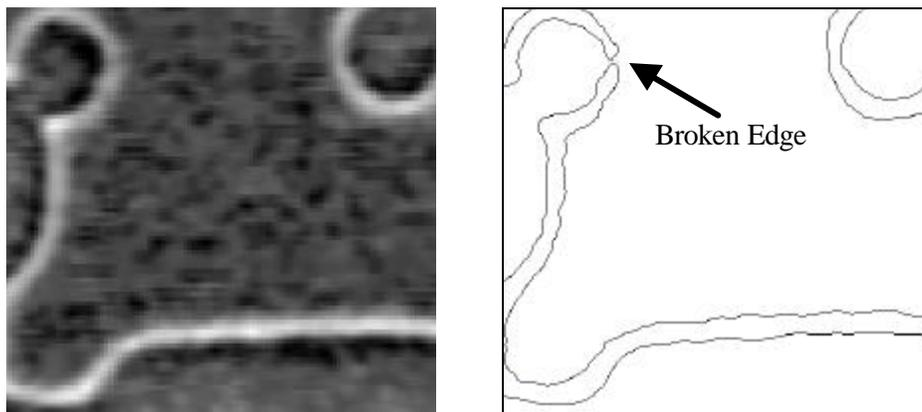
Figure 5. Broken edges are a common problem for images with low contrast edges.
