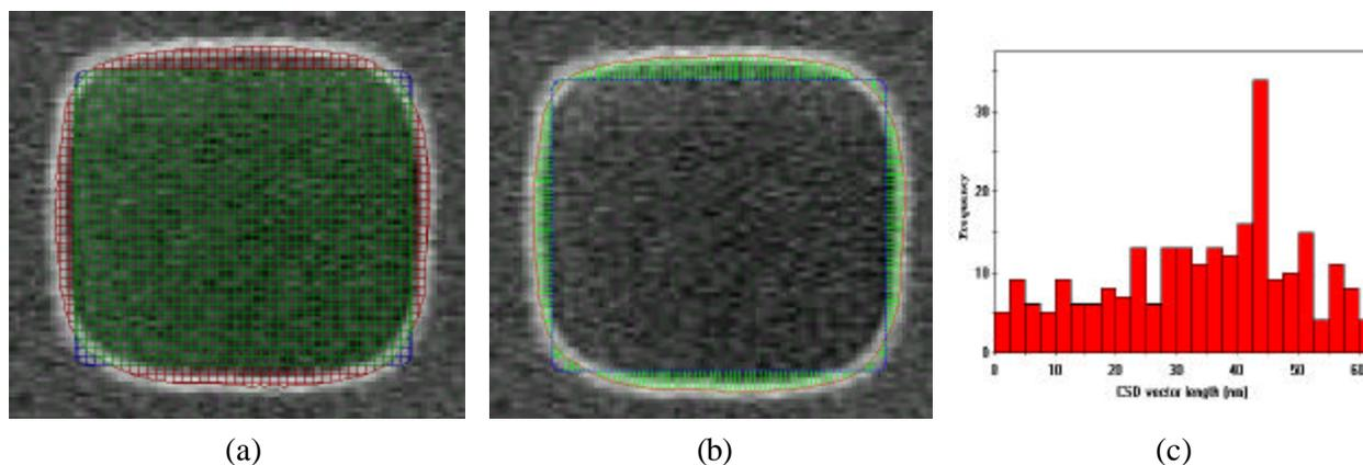
Figure 11. Analysis of overlapping critical shapes, such as this design to reticle comparison, can be used to calculate (a) overlapping areas, and (b) critical shape difference vectors, resulting in (c) a histogram of critical shape difference vector lengths.
