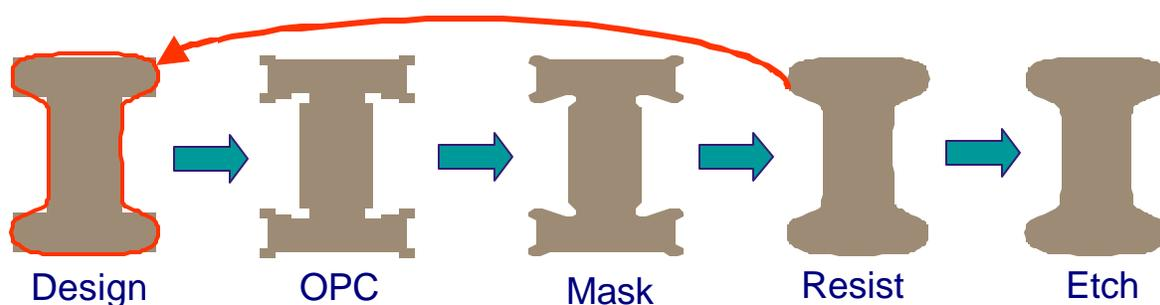
Figure 10. The comparison of a resist critical shape to the original design is one example of how critical shapes can be analyzed.
