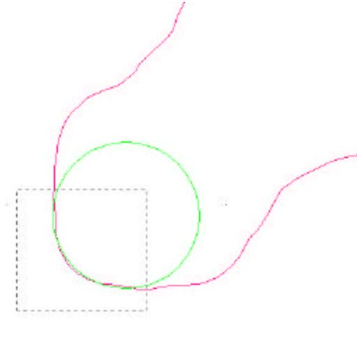
Figure 8. Corner rounding measurement where a circle is fit to the critical shape in a selected region.
