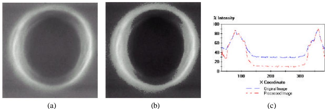
Figure 2. The impact of automatic gray level scaling: (a) original image, (b) after automatic gray level scaling, and (c) a horizontal line scan through the middle of the image showing gray levels both before and after scaling.
