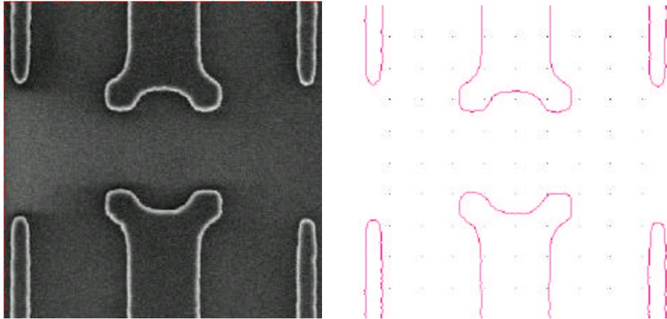
Figure 6. A typical 8250R SEM image of a chrome on glass reticle and the resulting critical shapes.
