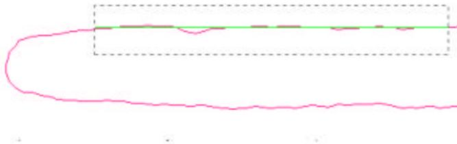
Figure 7. Line edge roughness calculations by fitting a straight line through a nominally straight edge.
