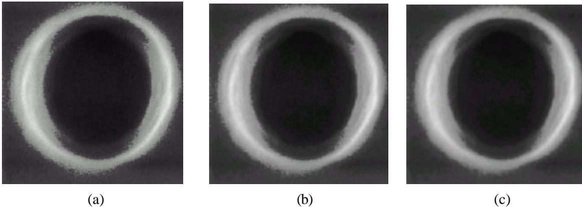
Figure 3. SEM images with (a) zero, (b) one, and (c) three passes of pixel smoothing.
