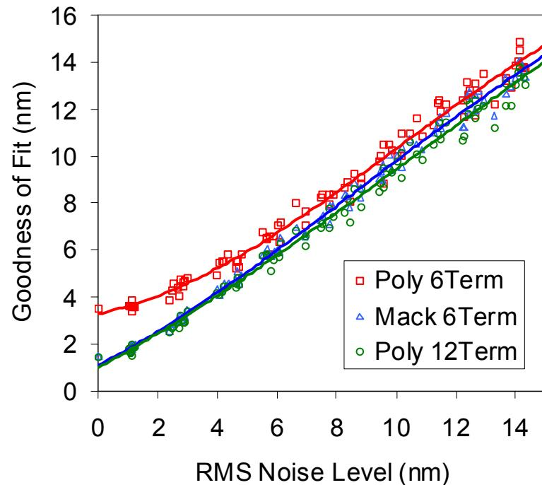
Figure 4. Comparison of goodness of fits for the various fitting functions in the presence of noise added to the data.
