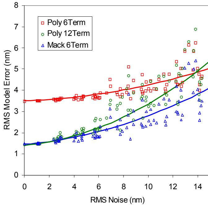
Figure 5. Behavior of the various fitting functions in the presence of added noise using the RMS model error as the metric to judge the effectiveness of each model at filtering noise.
