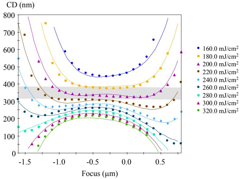
Figure 1. Example of the effect of focus and exposure on the resulting resist linewidth (symbols) and the best fit of this data (lines) to equation (1).
