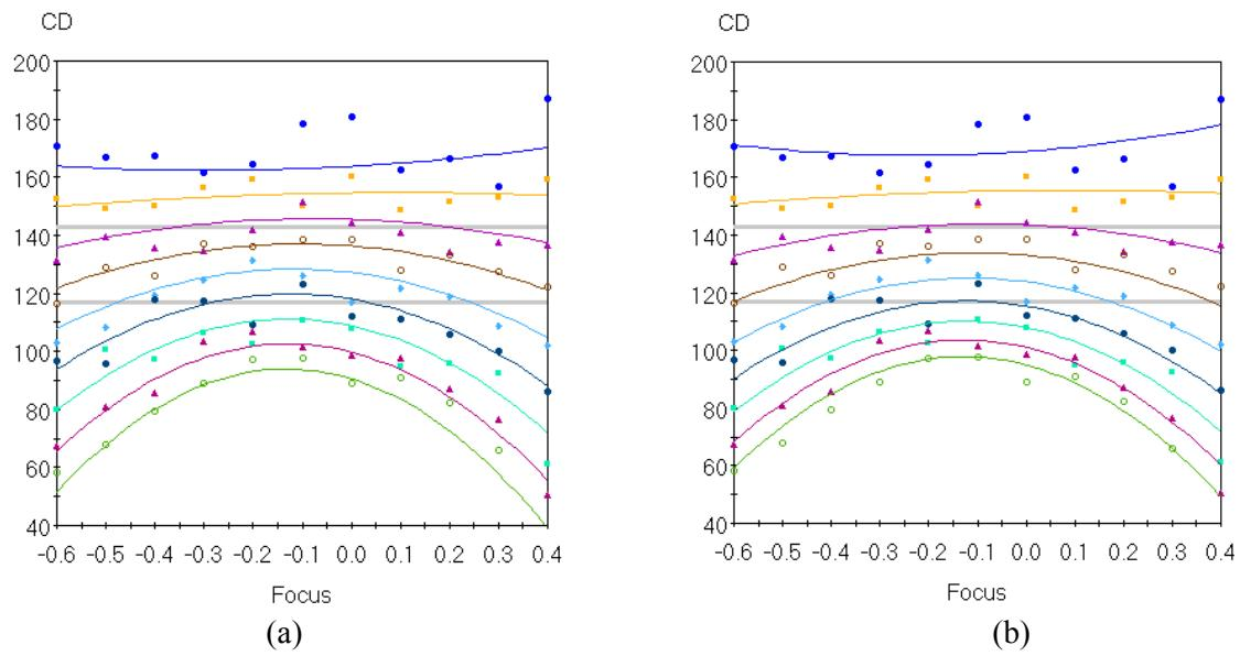
Figure 3. Comparison of the original polynomial (a) to the physically based fitting function (b) to data with 4.1nm RMS of added noise.
