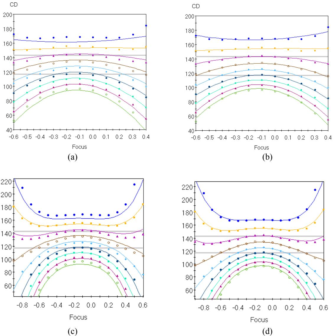
Figure 2. Comparison of the original (a and c) to the new (b and d) fitting function using the same number of terms in each expression and “noise free” data generated by simulation.
