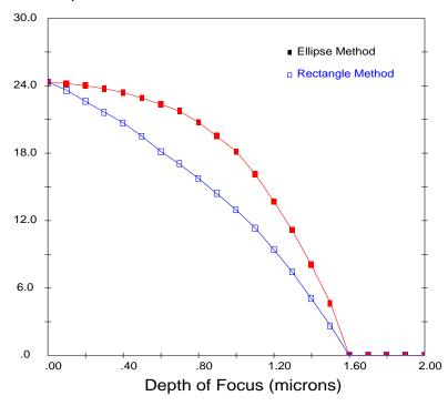
Figure 2. The process window of Fig. 1 is analyzed by fitting all of the maximum rectangles and all of the maximum ellipses, then plotting their height (exposure latitude) versus their width (depth of focus).
