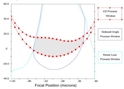
Figure 1. The focus-exposure process window constructed from contours of the specifications for linewidth, sidewall angle and resist loss. The shaded area shows the overall process window.
