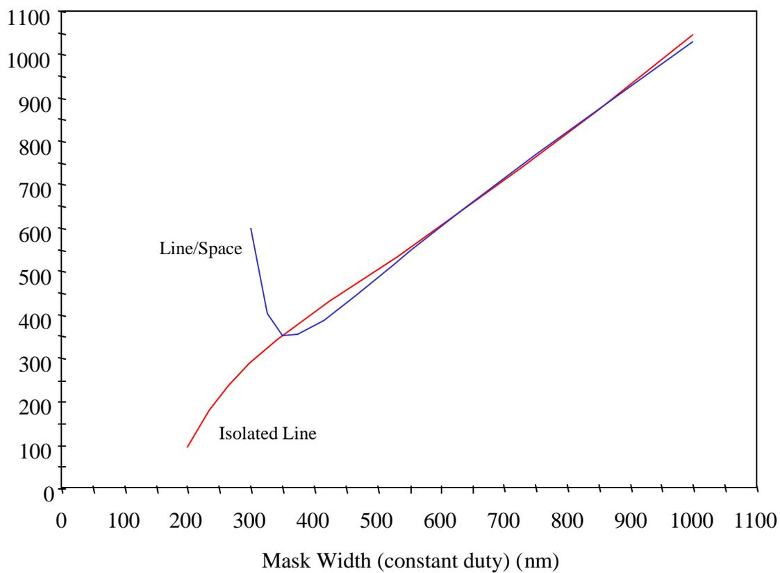
Figure 1. Typical mask linearity plot for isolated lines and equal lines and spaces (i-line, NA = 0.56,  $\sigma = 0.5$ ).
