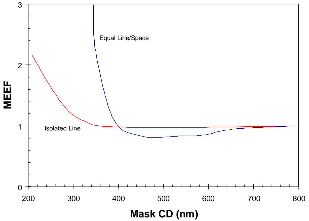
Figure 2. The mask error enhancement factor (MEEF) for the data of Figure 1.
