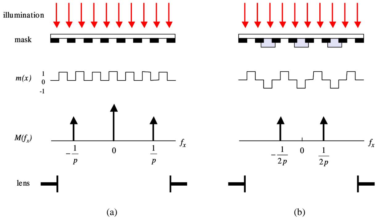
Figure 1. A mask pattern of lines and spaces of pitch  $p$  has an idealized amplitude transmittance function  $m(x)$  that produces a diffraction pattern  $M(f_x)$  where  $f_x$  is the spatial frequency. A binary chrome on glass mask is shown in (a), and an alternating phase shift mask is shown in (b).
