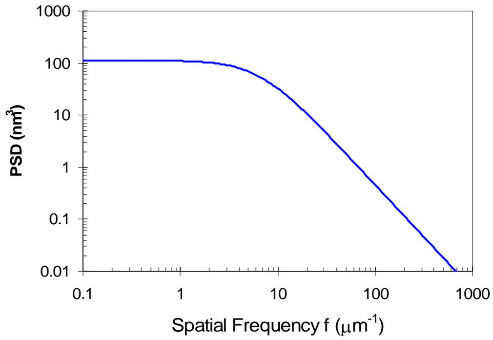
Figure 2. An idealized PSD with  $\sigma_{LER} = 1.5$  nm and  $L_c = 25$  nm.
