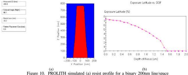
Figure 10. PROLITH simulated (a) resist profile for a binary 200nm line/space feature using CD-26 developer (diluted to 0.195N) at 35°C, and (b) Exposure Latitive vs. DOF analysis of a Focus-Exposure Matrix
