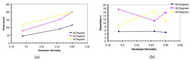
Figure 8: Plots of (a) the maximum dissolution rate  $R_{max}$ , and (b) the dissolution selectivity parameter *n* versus developer normality for different developer temperatures. At higher temperatures the effect of the developer normality is diminished on  $R_{max}$  and is erratic on the dissolution selectivity parameter *n*.
