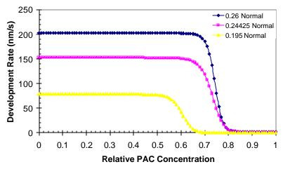
Figure 7: Comparison of the effect of developer normalities on the development rate of APEX-E at 35°C developer temperature. Shows the effects of decreasing maximum dissolution rate  $R_{ma}$ , and shift in  $m_{TH}$
