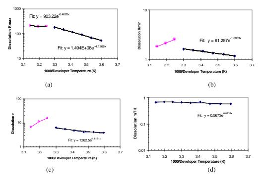
Figure 5. Arrhenius plots of (a) the maximum dissolution rate  $R_{max}$ , (b) the minimum dissolution rate  $R_{min}$ , (c) the dissolution selectivity parameter *n*, and (d) the threshold PAC concentration  $m_{TH}$ . Best fits to the Arrhenius equation are also shown.
