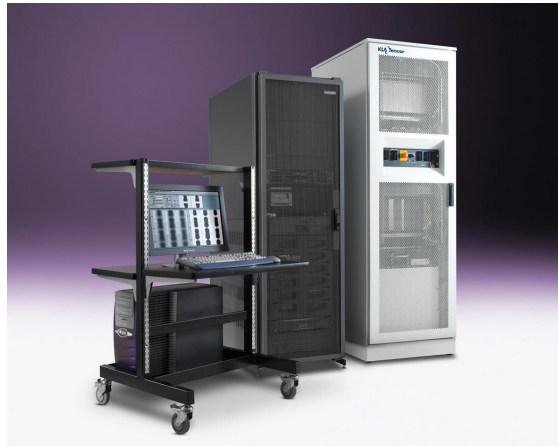
Figure 4: The DesignScan system hardware. The operator console is shown on the left. The TeraPrep sub-system is shown in the dark chassis and the image computer is shown on the right. A second operator console connected to the TeraPrep is not shown.
