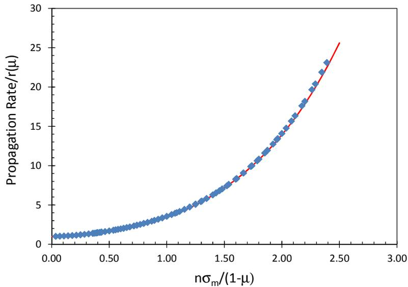
Figure 4. 3D simulation results for  $n = 10$ . Each data point is the average of between 4 and 50 trials.  $\mu$  was varied between 0.72 and 0.77 and  $\sigma_m$  was varied between 0.001 and 0.055. The resulting  $r(\mu)$  went from 0.08 to 1.92 nm/s, and the propagation rate varied from 0.1 to 6.7 nm/s.
