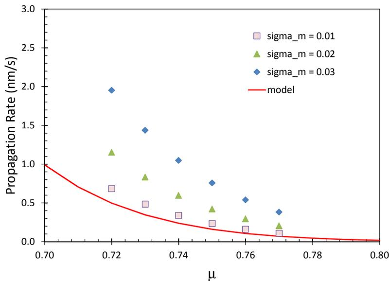
Figure 5. Comparison of 3D simulation results of the development front propagation rate (for  $n = 10$ ) for different  $\sigma_m$ . The “model” curve corresponds to  $\sigma_m = 0$ .
