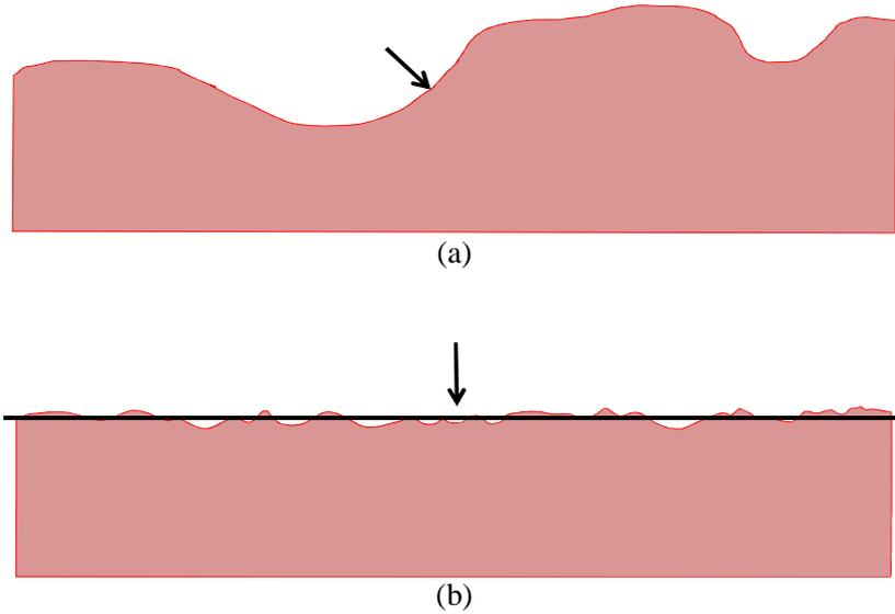
Figure 1. Photoresist development rate is defined in two ways: a) microscopic development – the rate at which a point on the resist surface moves perpendicular to that surface; and b) macroscopic development – the rate at which the mean surface position (the mean development front) propagates.
