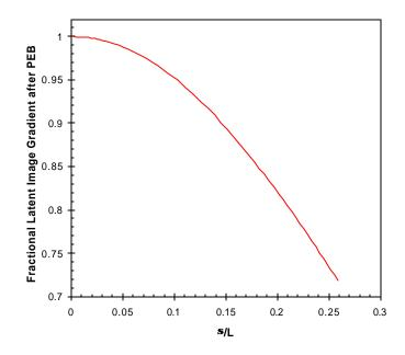
Figure 1. Increased diffusion (shown by the dimensionless quantity  $\sigma/L$ , the diffusion length over the width of the edge region) causes a decease in the latent image gradient after PEB.
