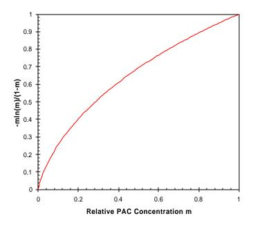
Figure 2. For a chemically amplified resist with an given required amount of amplification, the exposure dose (and thus relative sensitizer concentration m) is optimum as the dose approaches zero (m  $\rightarrow$  1).
