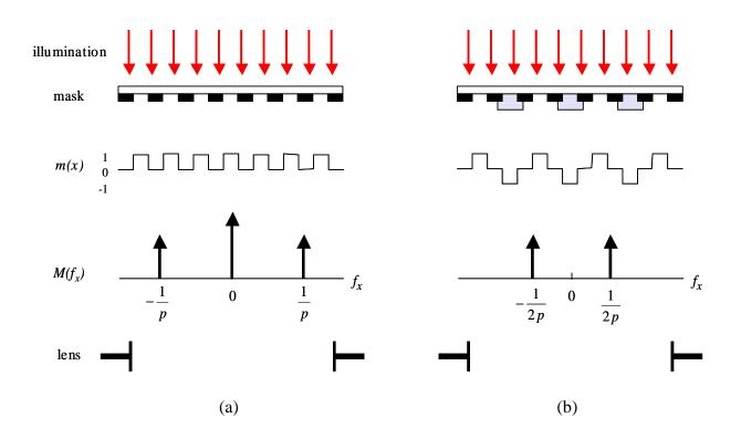
Figure 1. A mask pattern of lines and spaces of pitch p has an idealized amplitude transmittance function m(x) that produces a diffraction pattern  $M(f_x)$  where  $f_x$  is the spatial frequency. A binary chrome on glass mask is shown in (a), and an alternating phase shift mask is shown in (b).
