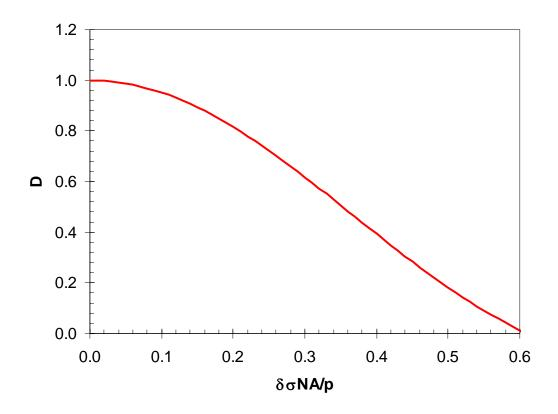
Figure 3. The Airy disk function D (which is linearly proportional to NILS) as it falls off with defocus.
