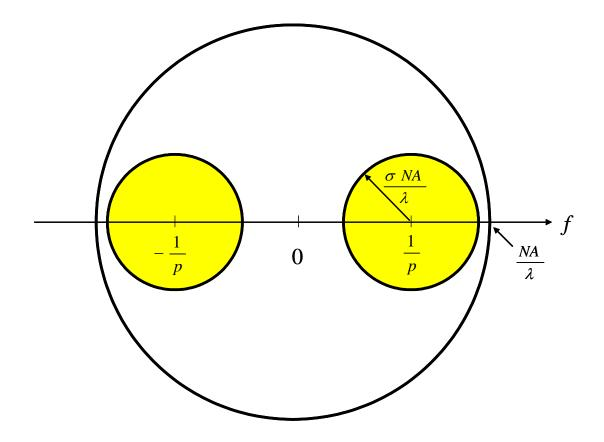
Figure 2. The diffraction pattern, spread out by a partially coherent source, for an alternating phase shift mask.
