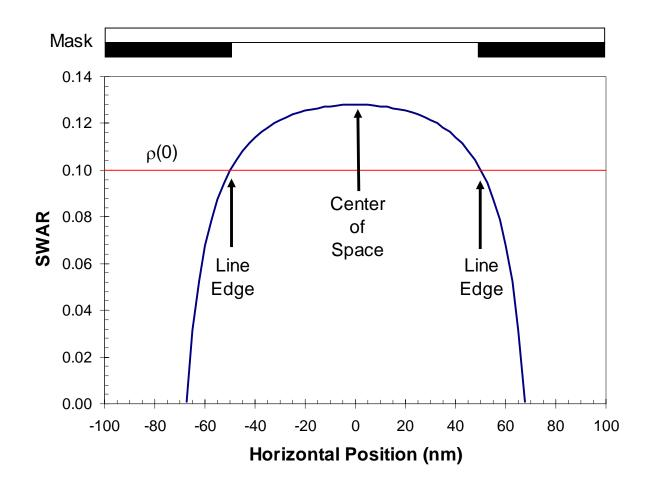
Figure 3. The standing wave amplitude ratio (SWAR) at different positions on the feature for threebeam imaging and *s*-polarization. For this example of three-beam imaging of 100nm lines and spaces,  $a_0 = 0.5$ ,  $a_1 = 0.3183$ ,  $|\rho(0)| = 0.1$ , and  $|\rho(\theta)| = 0.15$ .
